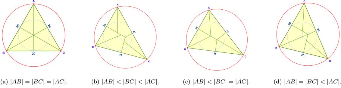
Figure 1: Case analysis for refining a triangle into six facets, triangles and quads, based on the relative length of  $AB$ . Voronoi edges (thick) lie on angle and edge-perpendicular bisectors (thin). Many edges are collinear.
