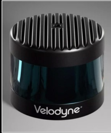
LIDAR (light detection and ranging) Velodyne VLS-128
