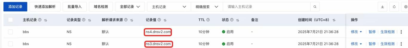
The screenshot shows the ACloud DNS Management console with the 'Host Record' table. Two NS records for the subdomain 'bbs' are listed, with their values 'ns4.dnsPod.com' and 'ns3.dnsPod.com' highlighted with red boxes.
