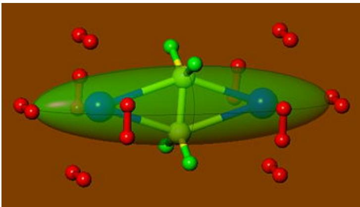
Results of modeling studies indicate that attaching titanium atoms (blue) to the ends of an ethylene molecule (yellow-green) will result in a capsule-shaped complex that absorbs 10 hydrogen molecules (red). The results open a new avenue in the pursuit of materials that will enable efficient solid-state storage of hydrogen. Credit: NIST
