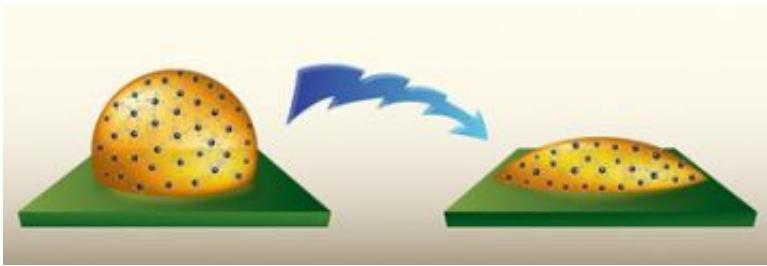
The contact angle of a droplet of nanofluid solution changes when exposed to an electric field. Image Credit: Rensselaer/Borca-Tasciuc
