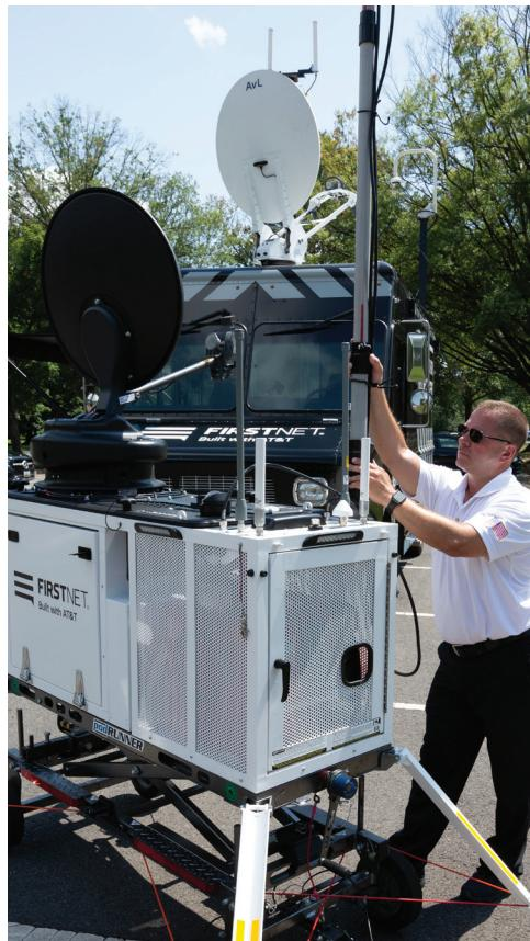
**Warning:** You can't simultaneously transmit FirstNet cellular from the CRD while FirstNet SIM cards are in the Cradlepoint router. Use FirstNet SIM cards only when providing Wi-Fi and/or wired Ethernet with the FirstNet cell tower radio off.
