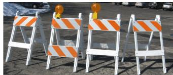
Barricades must be white with reflective tape across the wood plate at the top. Homemade devices, vehicles and/or other objects are not authorized in lieu of barricades. The minimum length for Type I and Type II Barricades is 24". Each barricade rail shall be 8" – 12" wide. A Type I panel has one (1) 8" x 24" retro-reflective panel per side, whereas a Type II barricade has two (2) 8" X 24" retro-reflective panels per side.
