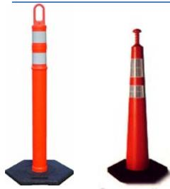
Delineators are commonly called candlestick cones and are used to channel vehicular traffic and should be placed no more than fifteen feet (15') apart. Delineators you use at your event must be a minimum of 21" high and must be high-speed roadway-quality cones. You must use traffic cones with reflective tape if they are used to support event plans in which environmental factors limit the visibility of their presence (e.g. fog, evening darkness, etc.)
